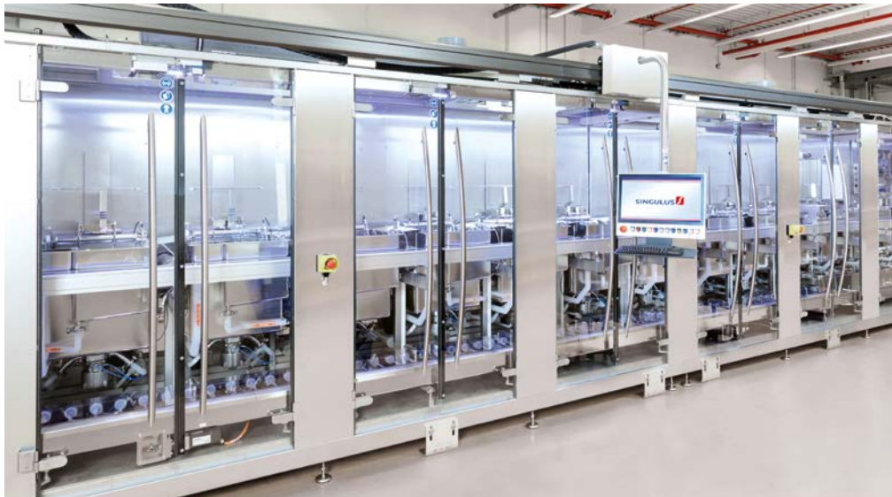
MEDLINE processing system for cleaning and deposition of disposable contact lenses.
