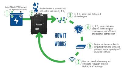
A HydraGEN TM unit also provides additional features. It is linked via Bluetooth to the driver's cell phone, updating in real time precious fleet-management data through the MyHydraGEN TM Technology App. All the data gathered by HydraGEN TM data is uploaded into the cloud, enabling the fleet manager to access it remotely in real time. The driver also receives an alert on his phone when the distilled water level is running low and
